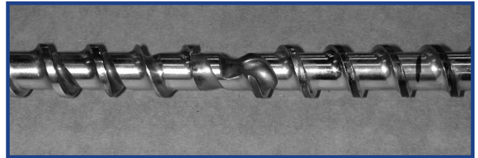
Severe Abrasive Wear
